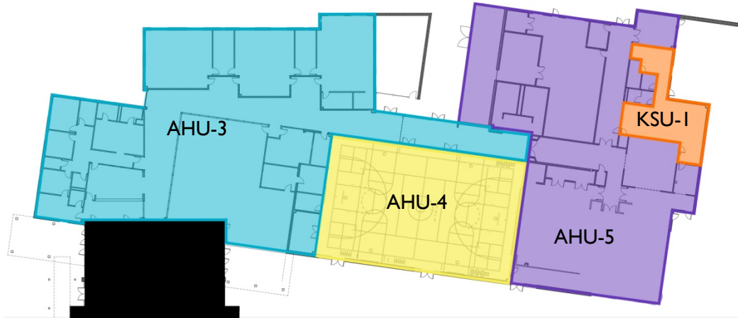
Figure 2: Wing B AHU Distribution
